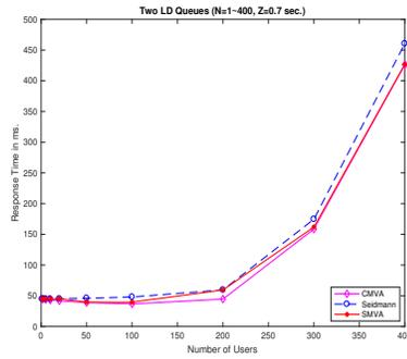
**Fig. 11** Response time with  $Z=0.7$  seconds
